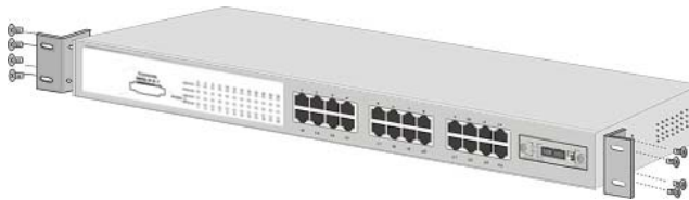
Figure 2-5. Attach mounting brackets with screws
